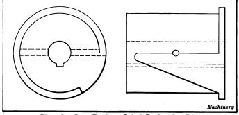
Fig. 16. Cam Used on Spiral Perforating Die
